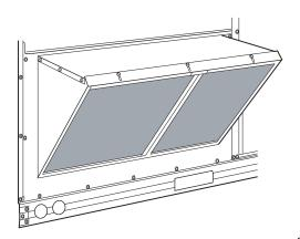
C07156 Fig. 4 - Screens Installed on Outdoor-Air Hood (Sizes 7-1/2 to 12-1/2 Tons Shown)
